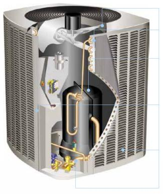
**Precision-Balanced Direct-Drive Fan –** Delivers quiet operation.
