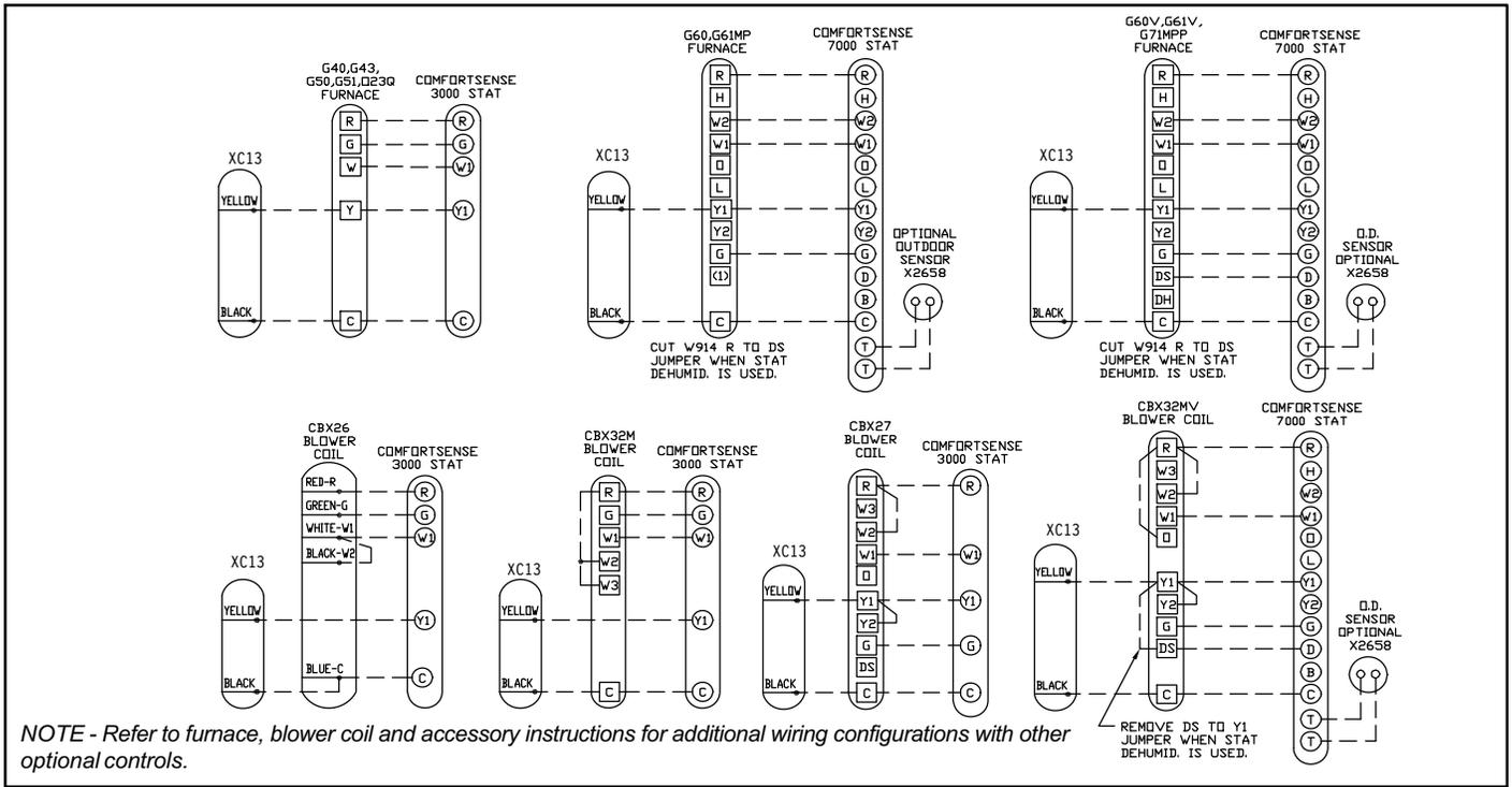
Figure 14. 24VAC Control Wiring Diagrams (Field Installed)
