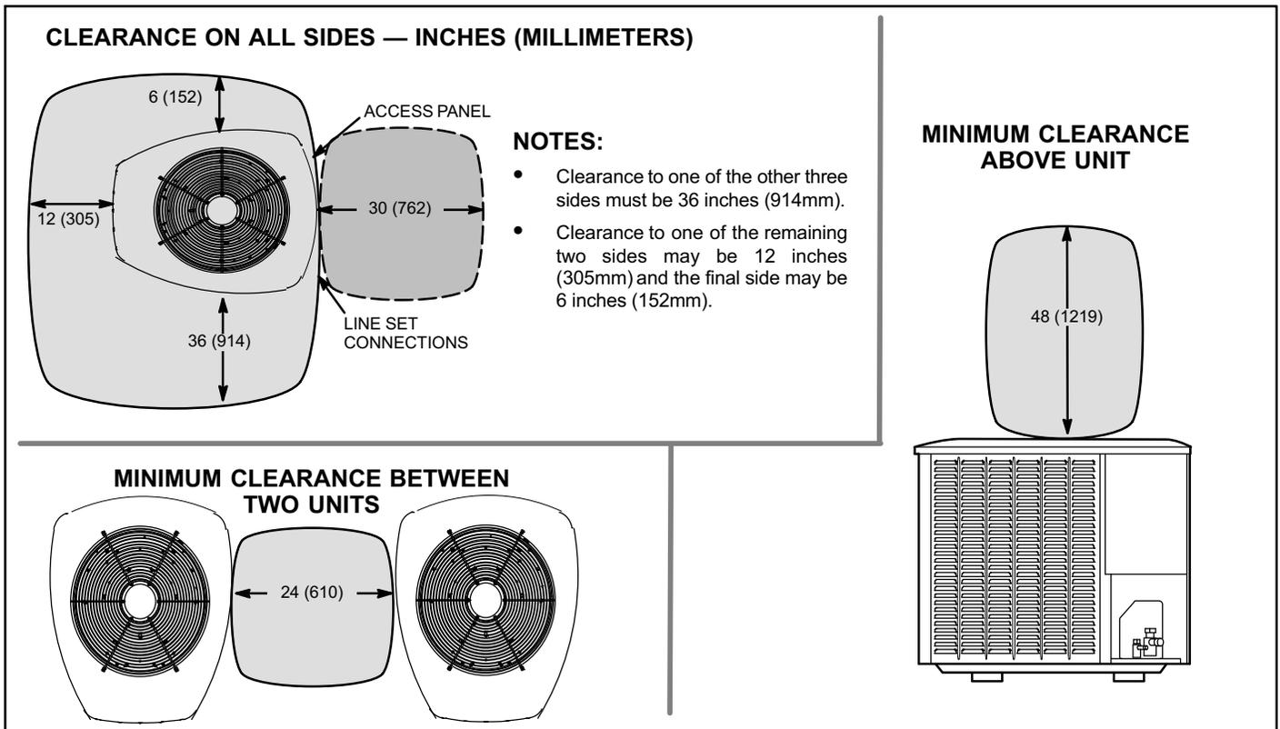
Figure 4. Installation Clearances
