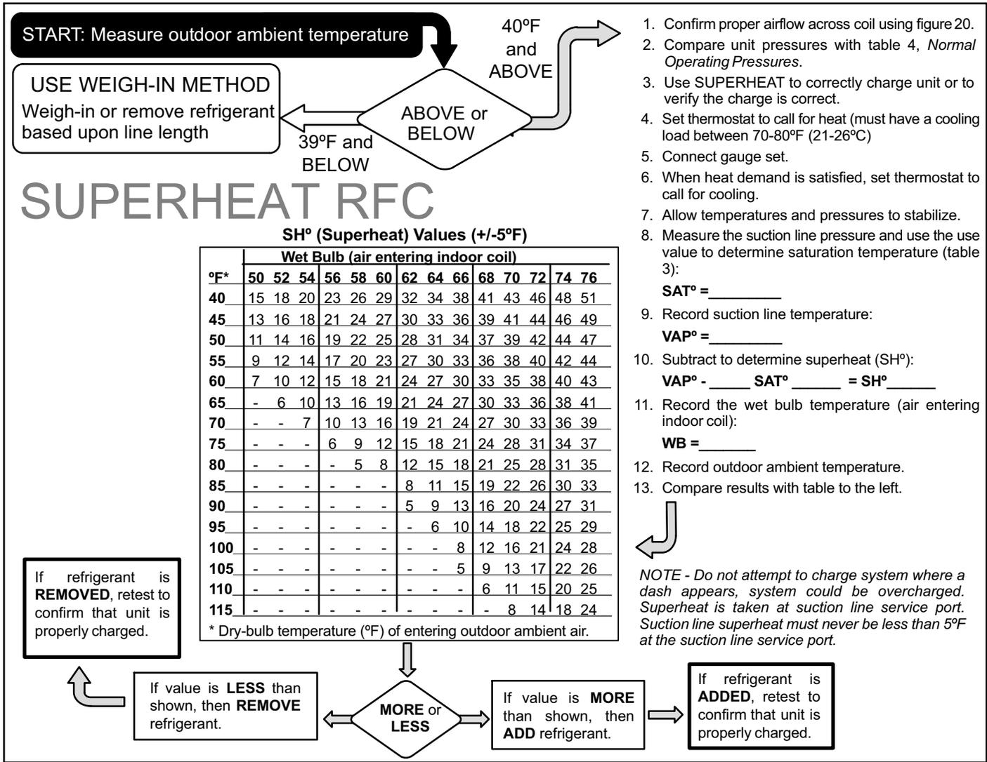
**Figure 24. Using HFC-410A Superheat (Fixed Orifice) Charge Method**
