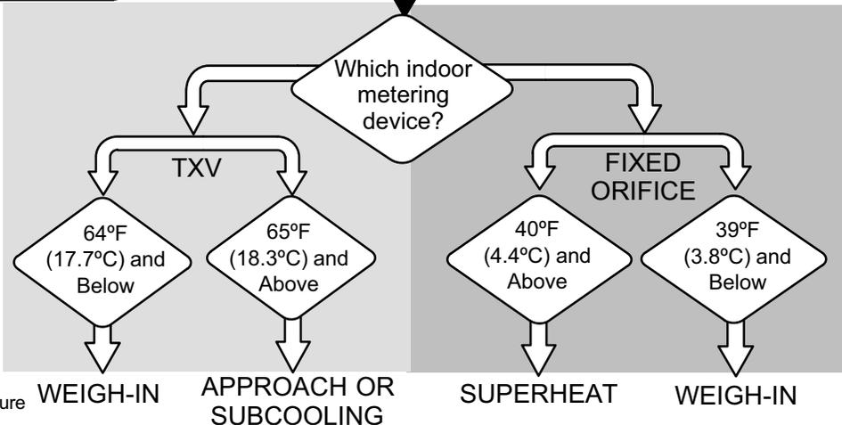
**Figure 19. Determining Charge Method**
