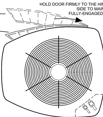
**IMPORTANT!** DO NOT ALLOW PANELS TO HANG ON UNIT BY TOP TAB. TAB IS FOR ALIGNMENT AND NOT DESIGNED TO SUPPORT WEIGHT OF PANEL.
