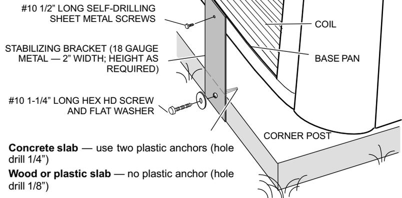
**Concrete slab** — use two plastic anchors (hole drill 1/4")
