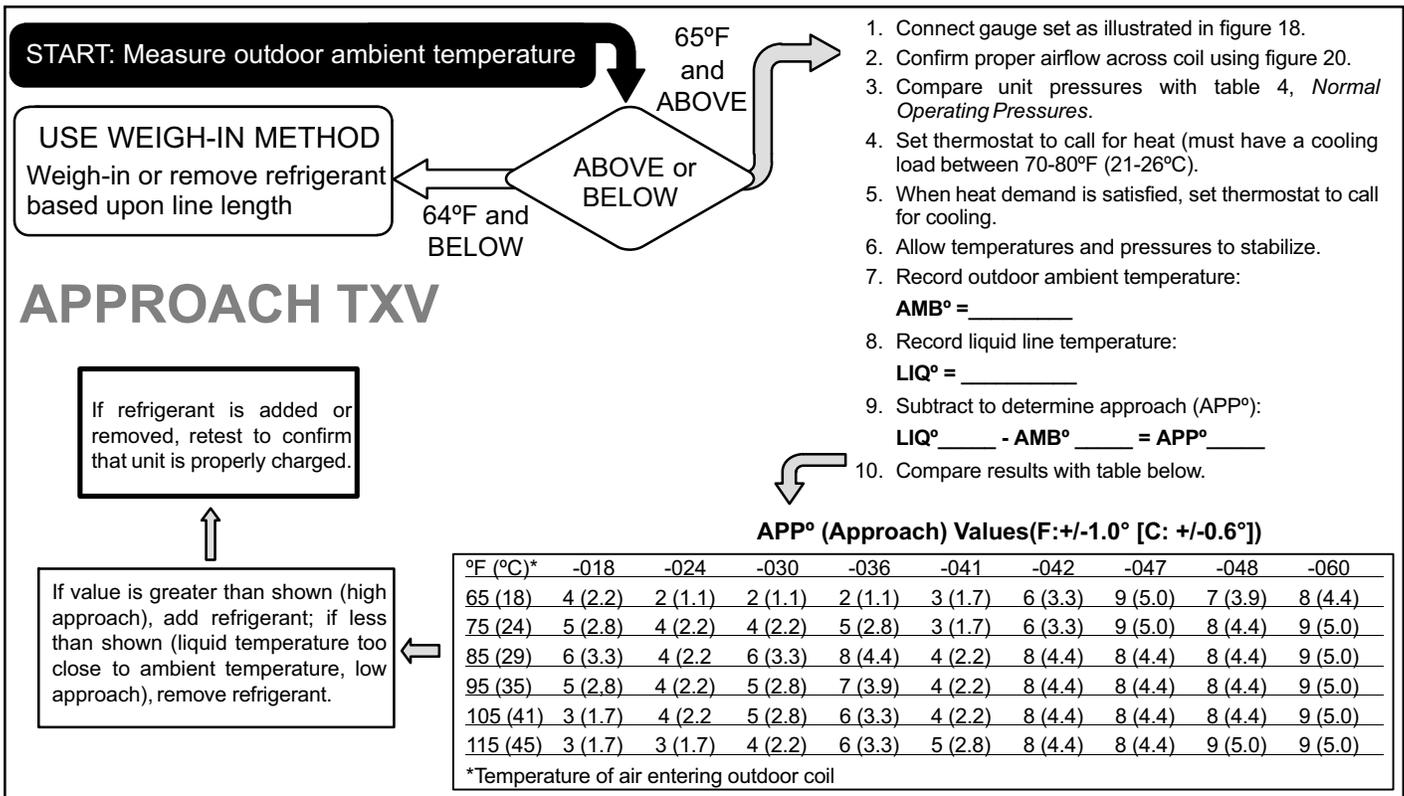
Figure 22. Using HFC-410A Approach (TXV) Charge Method
