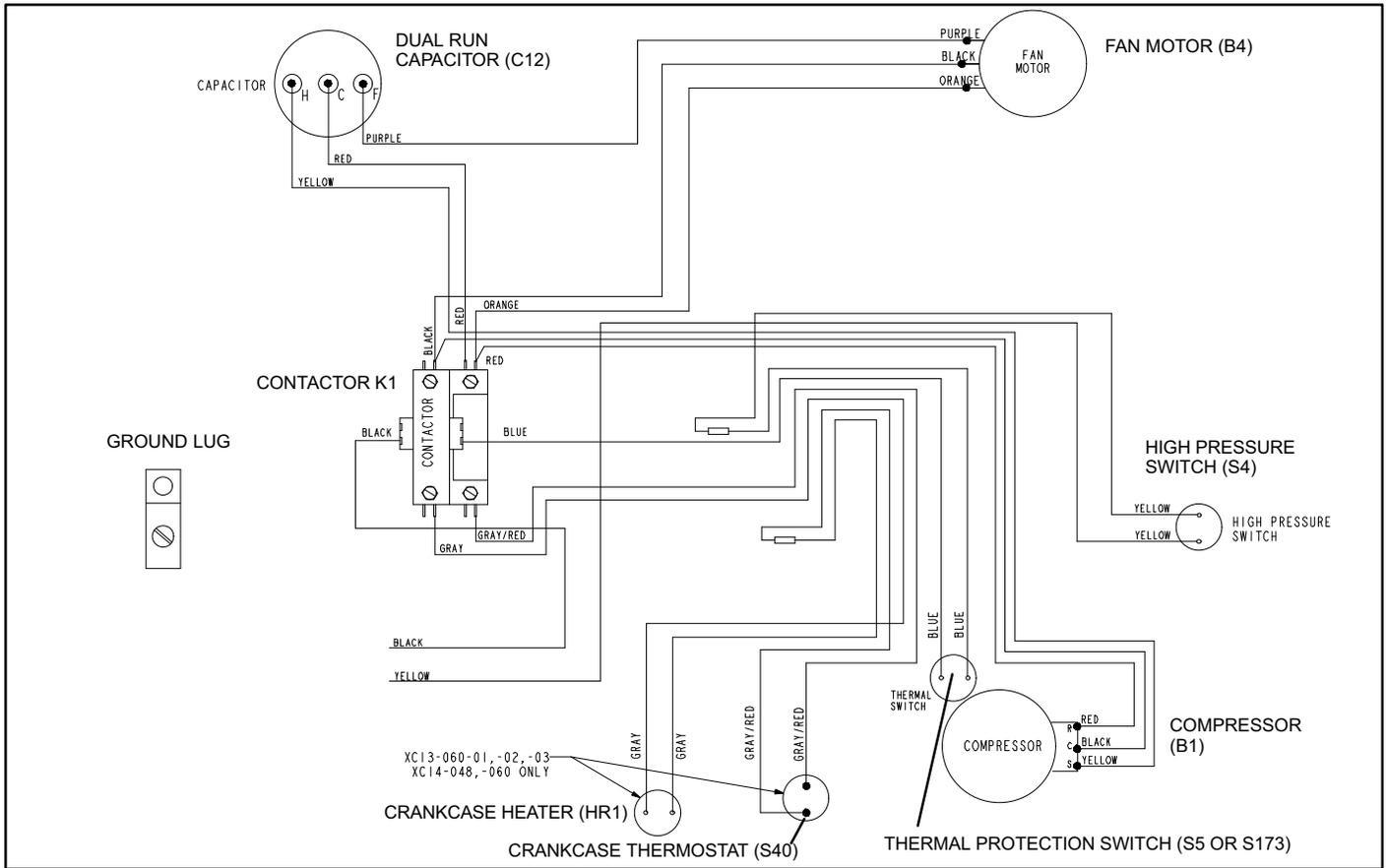
**Figure 16. Typical Factory Wiring Diagram (Interlink Compressor)**
