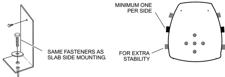
One bracket per side (minimum). For extra stability, two brackets per side, two inches (51mm) from each corner.
