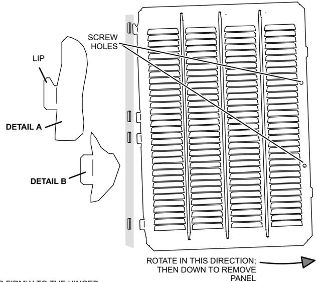
Figure 6. Removing and Installing Panels
