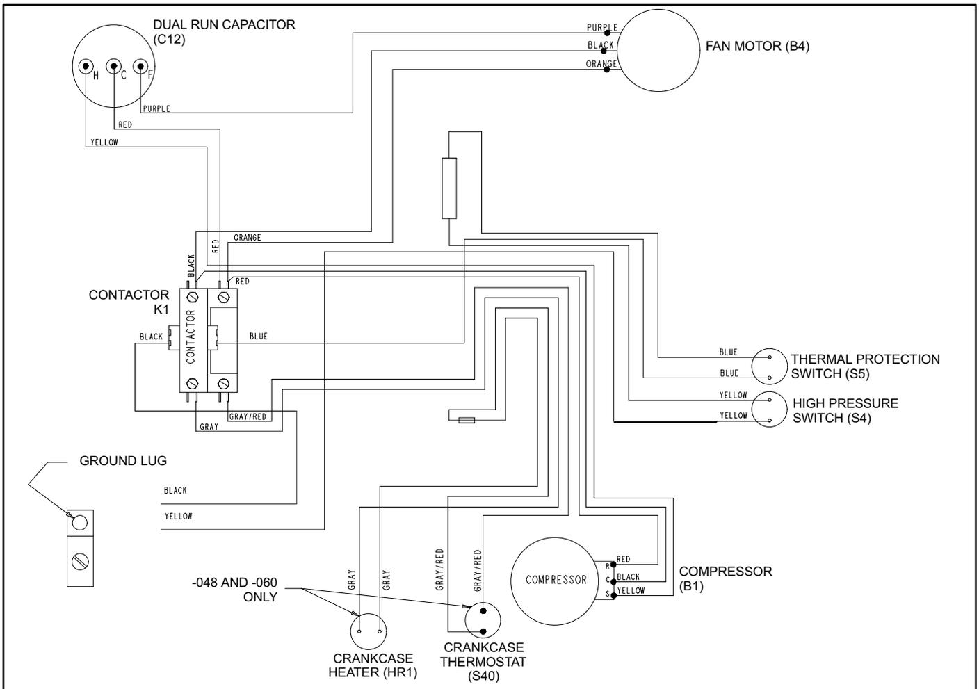
Figure 15. Typical Factory Wiring Diagram (Copeland Compressor)
