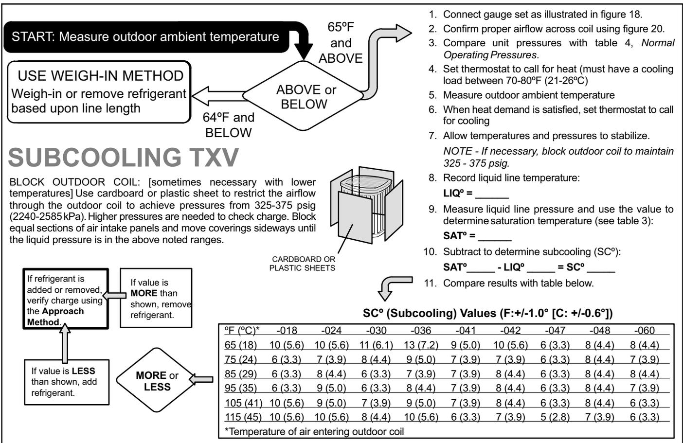
Figure 23. Using HFC-410A Subcooling (TXV) Charge Method
