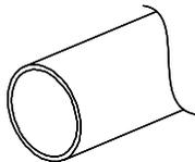
Cut ends of the refrigerant lines square (free from nicks or dents). Deburr the ends. The pipe must remain round, do not pinch end of the line.
