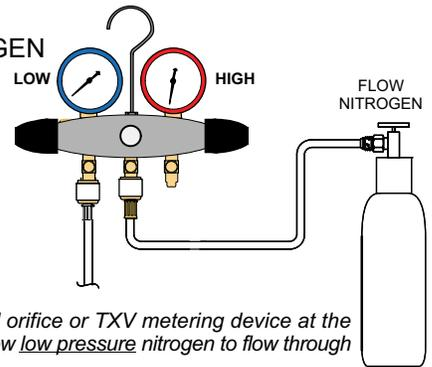
**NOTE** - The fixed orifice or TXV metering device at the indoor unit will allow low pressure nitrogen to flow through the system.
