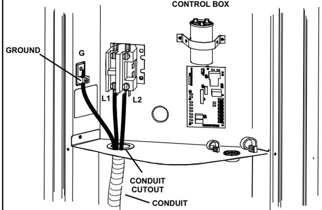
**NOTE - Any excess high voltage field wiring should be trimmed and secured away from any low voltage field wiring.**
