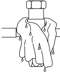
To protect components during brazing, wrap a wet cloth around the liquid line service valve body and copper tube stub and use another wet cloth underneath the valve body to protect the base paint. Also, shield the light maroon R-410A sticker.
