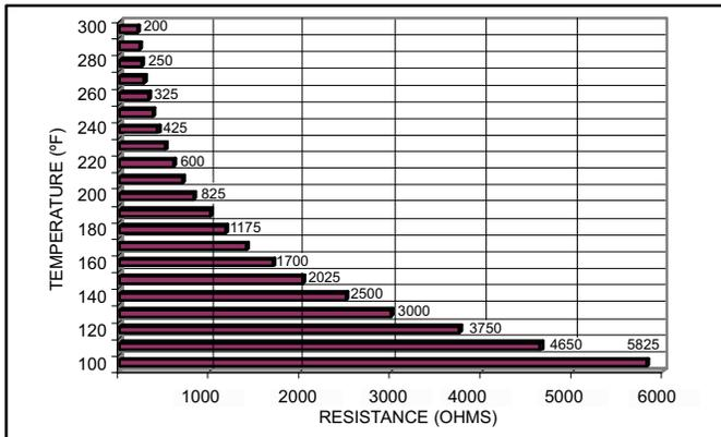
**Figure 36. Temperature/Resistance Chart (Discharge Sensor)**
