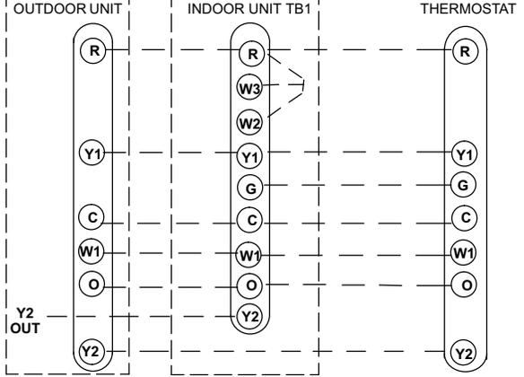
Install low voltage wiring from outdoor to indoor unit and from thermostat to indoor unit as illustrated.
