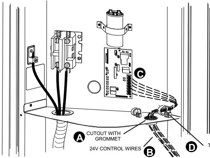
— HIGH VOLTAGE FIELD WIRING
