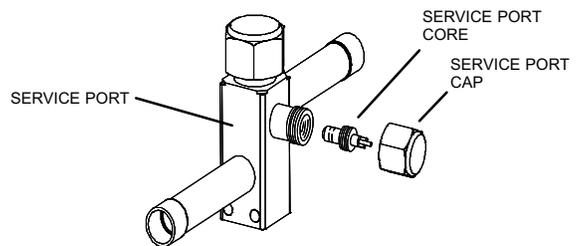
After all connections have been brazed, disconnect manifold gauge set from service ports, cool down piping with wet rag and remove all wrappings. Do not reinstall cores until after evacuation procedure. Reinstall service caps if desired to close off refrigerant ports.
