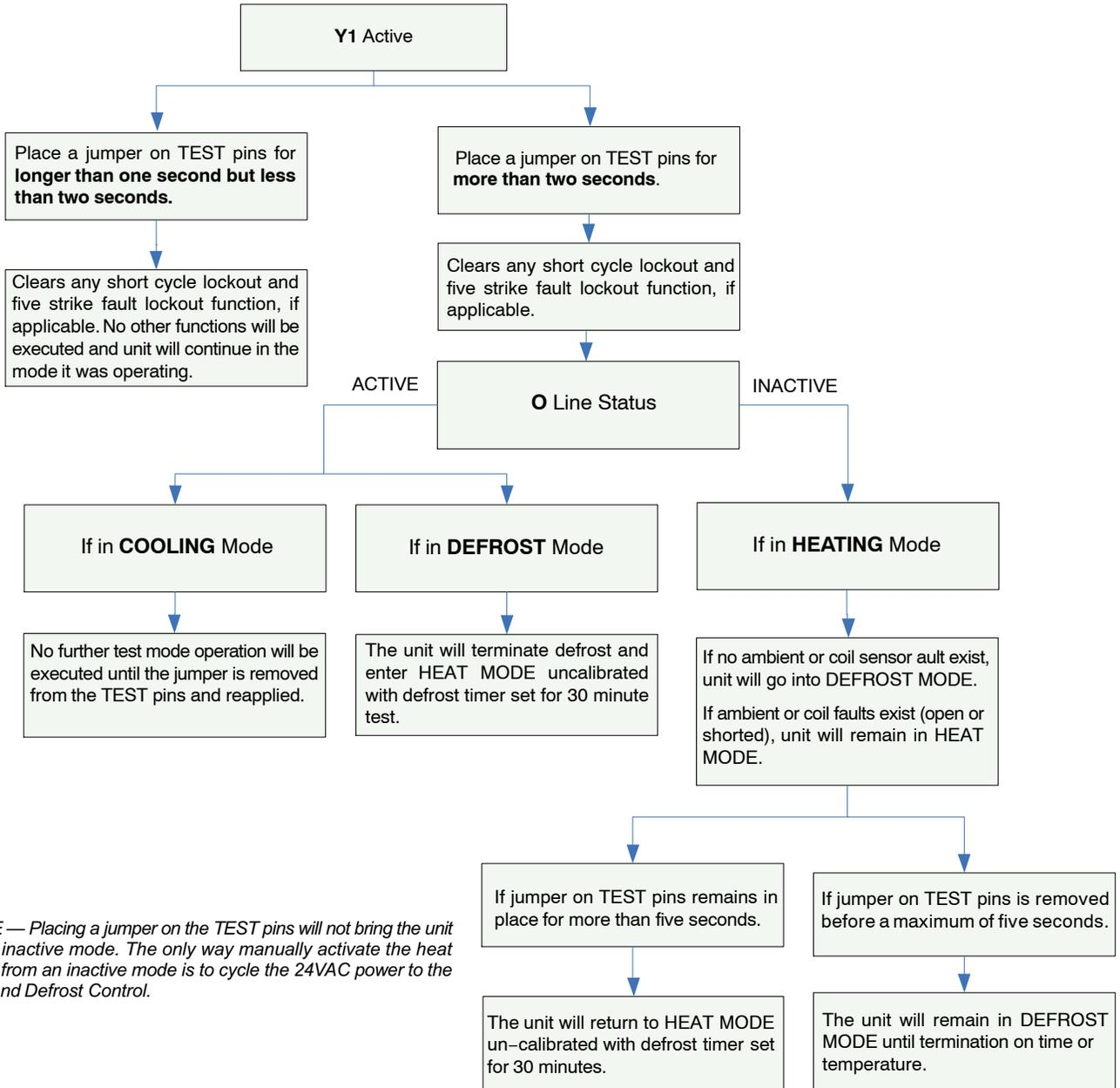
**NOTE** — Placing a jumper on the TEST pins will not bring the unit out of inactive mode. The only way manually activate the heat pump from an inactive mode is to cycle the 24VAC power to the Demand Defrost Control.
