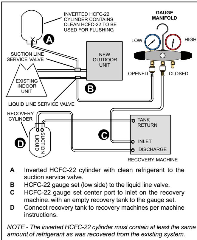
Figure 19. Typical Flushing Connection
