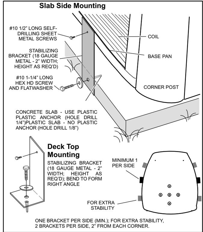
**Figure 13. Installing Stabilizer Brackets**
