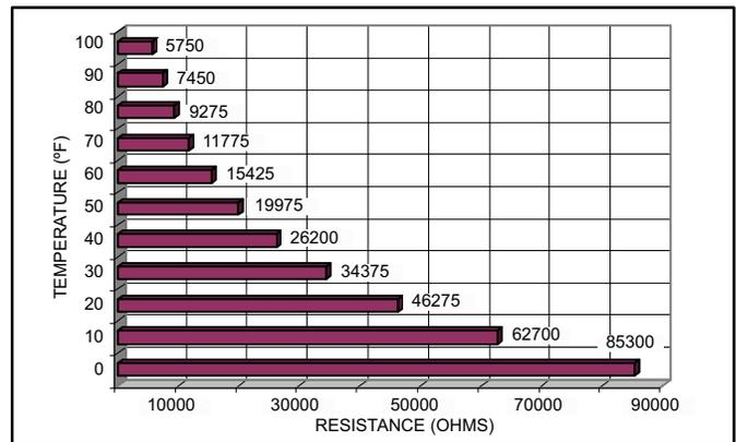
**Figure 34. Temperature/Resistance Chart (Ambient and Coil Sensors)**
