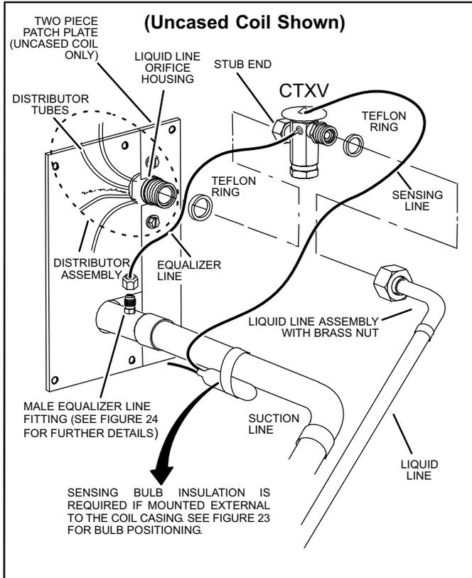
**Figure 22. Typical CTXV Installation**
