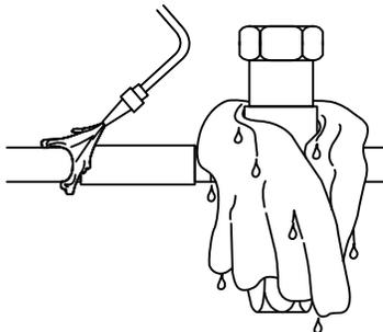
Braze the liquid line to the liquid line service valve. Turn off nitrogen flow.
