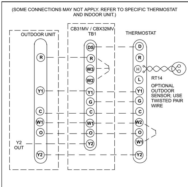
Figure 28. Outdoor Unit and CB31MV/CBX32MV Thermostat Designations
