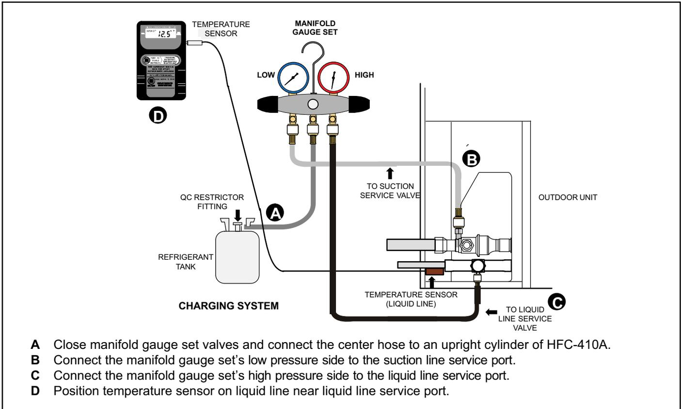
Figure 29. Connecting Gauge Set for Testing and Charging
