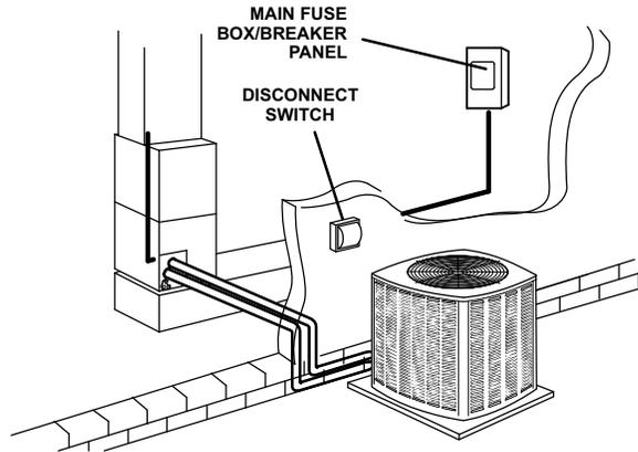
Refer to the unit nameplate for minimum circuit ampacity, amperage minimum, and maximum fuse or circuit breaker fusible (HACR per NEC). Install power wiring and properly sized disconnect switch.
