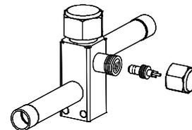
Remove service cap and core from both the suction and liquid line service ports.
