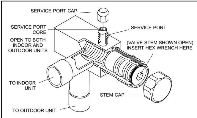
**Figure 4. Angle-Type Service Valve (Back-Seated Opened)**
