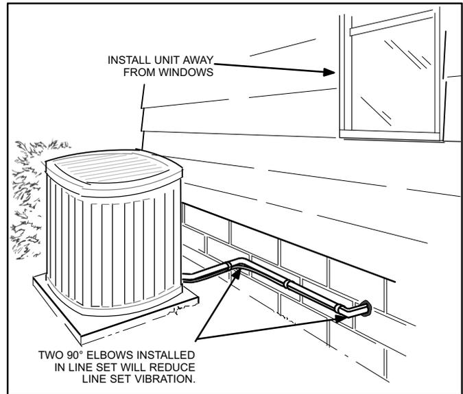
Figure 7. Outside Unit Placement
