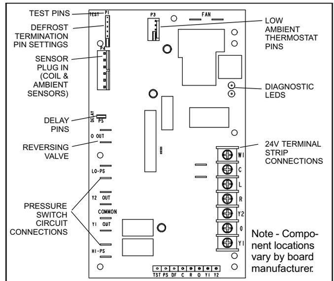
**Figure 33. Defrost Control Board**
