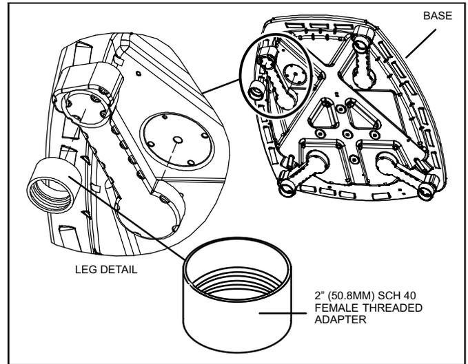
**Figure 10. Elevated Slab Mounting using Feet Extenders (Larger Base Units)**
