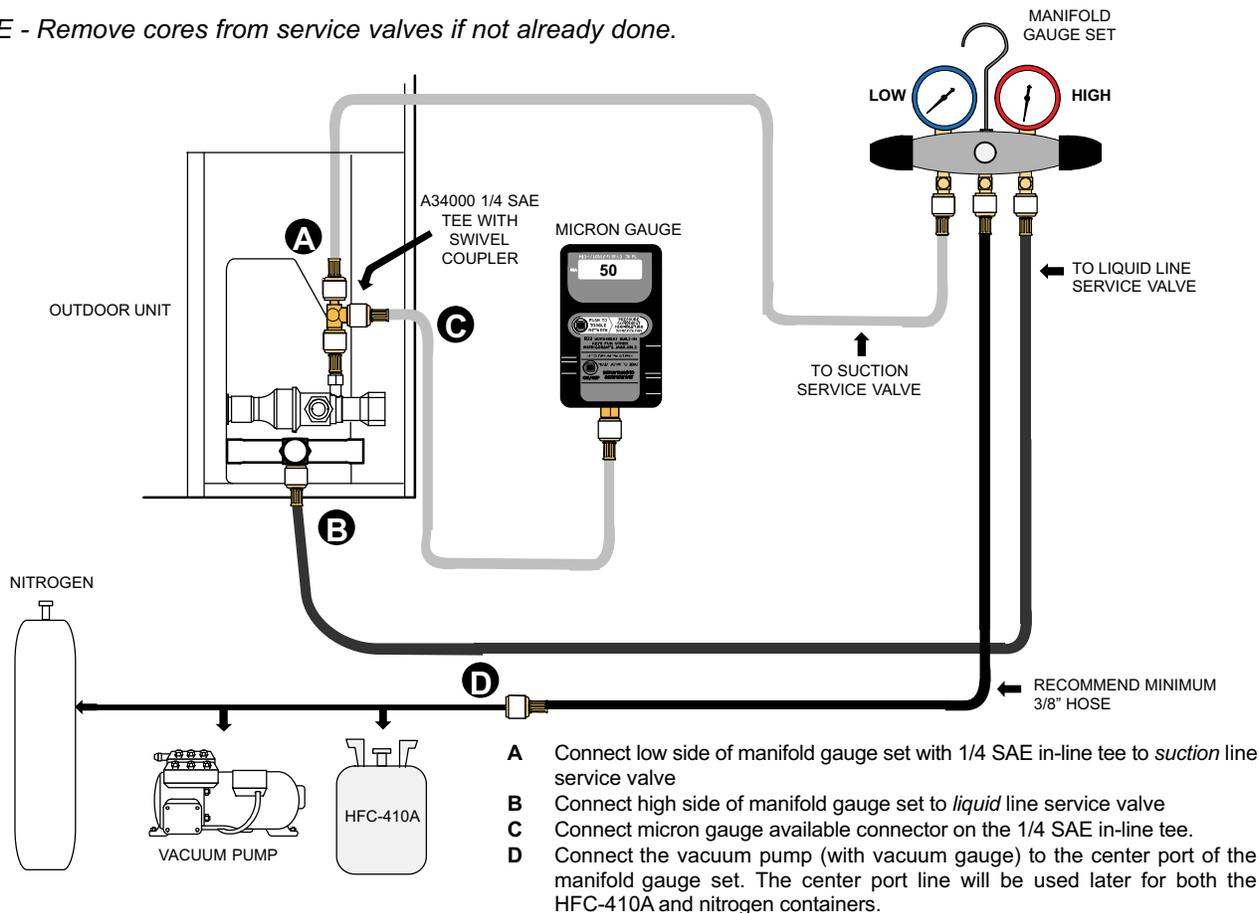
Figure 26. Typical Evacuation Manifold and Micron Gauges Connections
