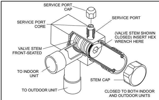
**Figure 3. Angle-Type Service Valve (Font-Seated Closed)**
