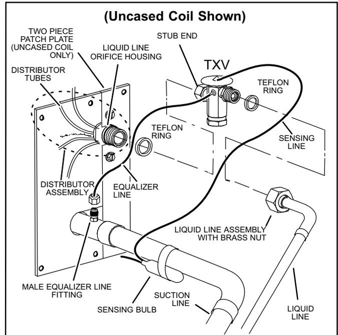
Figure 18. Typical TXV Removal
